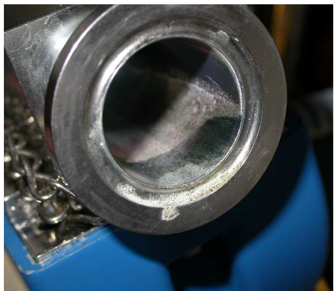
Figure 11 Rouging inside the HPLG cell after the test involving artificial rouge formation. Loose particles may be wiped off the surface
