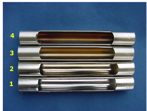
Figure 1 Tube inserts representing different degrees of rouging. The tubes measure: 162 x 21.8 x 1.5 mm (length x outer diameter x wall thickness)
